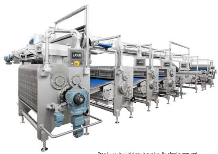
Once the desired thickness is reached, the sheet is engraved and cut by a **rotary cutting machine** and thousands of biscuits are formed every minute. The scraps are automatically recovered and taken back to the hopper of the initial extruder to be reused together with the fresh mixture. Once cut, the biscuits can be decorated with sugar, seeds or glazes before entering the baking phase. All this takes place automatically and without the need for direct intervention by operators.
